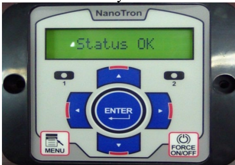
Figure 7: The phrases, "Status OK" and "Initializing", will cycle on the display for approximately one minute.
