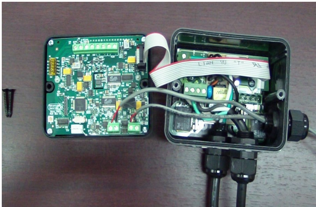
Figure 1: The logic board on back side of faceplate of NANO-M
