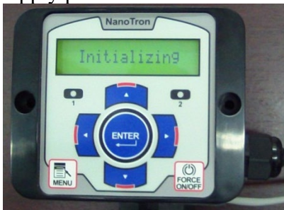
Figure 3: The LCD display will illuminate, and a startup sequence will commence upon power up. When the 'Initializing' message appears on the display, the NANO-M is ready for user interaction.
