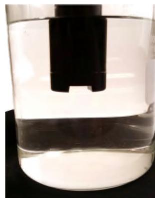
***IMPORTANT NOTE: MAKE SURE TO REMOVE ALL BUBBLES FROM THE OPTICAL FACE BY TILTING THE LITTLE DIPPER™ 2 AND GENTLY SHAKING WHILE FULLY SUBMERGED IN THE WATER AS AIR BUBBLES TRAPPED NEAR OR ON THE OPTICAL HEAD WILL INFLUENCE RESULTS.***
