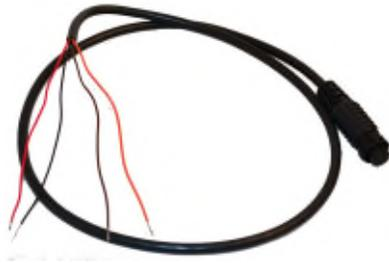
When connecting the Little Dipper 2 to the cable, pay special attention to the orientation of the pins. Once the connection is made, slide the collar down and rotate the collar to secure.
